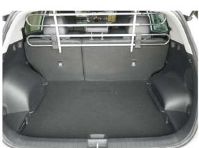
When the false floor is lowered it slopes down from behind the rear seats
